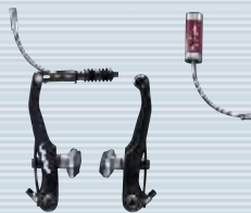
POWER MODULATOR (SM-PM40) и V-BRAKE
